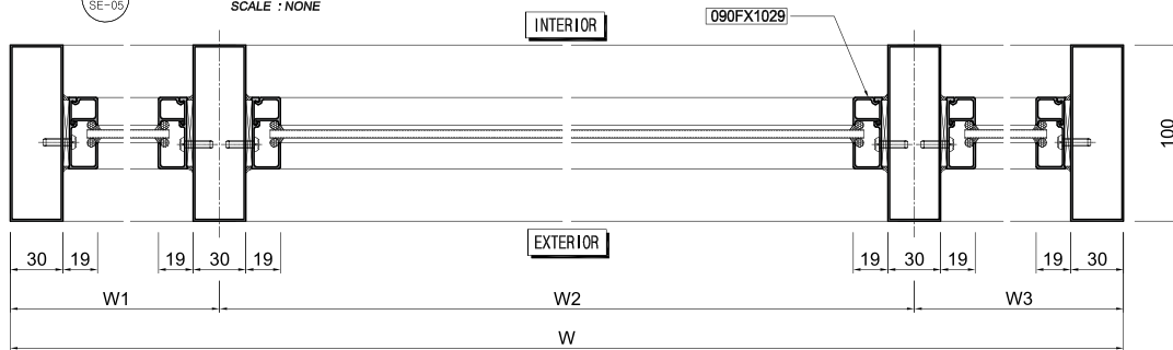
2 SE-05 Horizontal Section Detail SCALE : NONE
